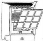
4. Replace the Filter Assembly, inserting the bottom of the Filter Assembly first.
