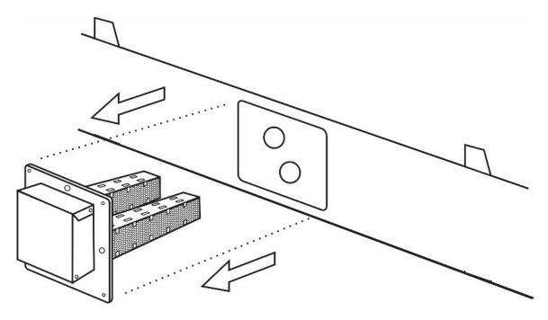
• Remove the two bolts on either side of the cell to remove the cell from the ballast assembly
