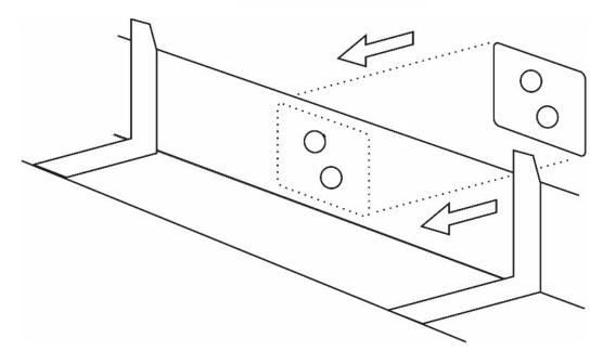
• Place the mounting plate squarely into place and fasten to duct work with metal screws.
